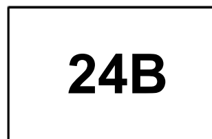
24B= Device code Marking (Top View)
